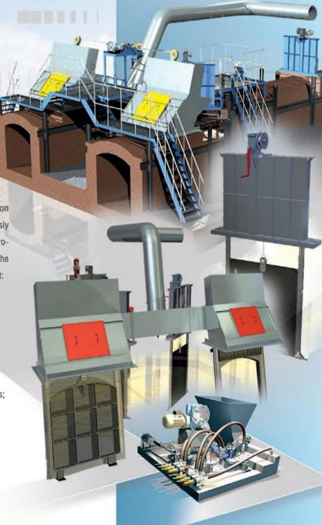
The glass mass scraper granulator produced by "Stromizmeritel" Closed JSC consists of a metal case, made of several sections attached together, inside of which is a chain conveyor, consisting of two
