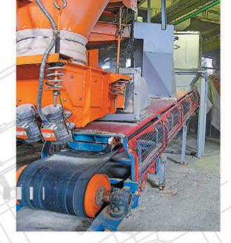
Belt conveyors are the most commonly used means of continuing transport, intended for moving different bulk goods with a wide range of various properties.
