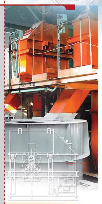
The vertical belt-type bucket elevators are used for lifting of various free-flowing and bulk materials from the loading point to the unloading point.
