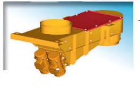
The installation of shut-off rotary gate valves on the vibrating loading and unloading feeders of the weighing dosing devices increases the accuracy of dosing and prevents the material falling from a conveying tray after the drive has been switched off. Equipment of the vibrating feeders with a sorting grid allows to separate preliminary small faction when feeding glass cullet into a crusher what essentially reduces load on the operating crusher and increases its service life.
